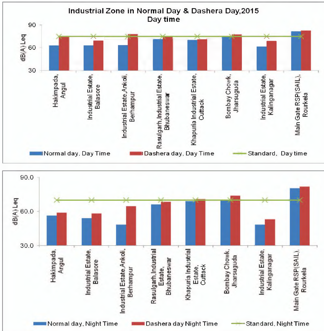
Fig. 8.4 Day time and Night time Noise Levels during Dashera in Industrial Zones (2015)
