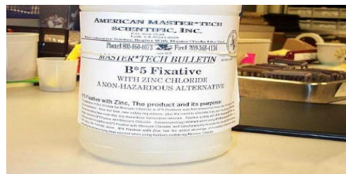
Figure (24) B-5 Fixative has been developed using zinc chloride in place of mercury.
